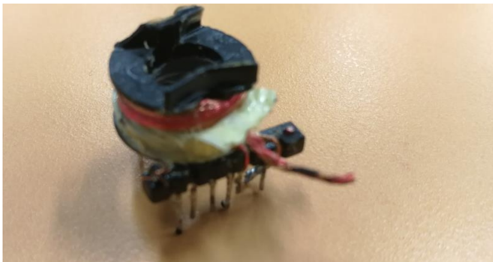
Overall view of secondary winding
