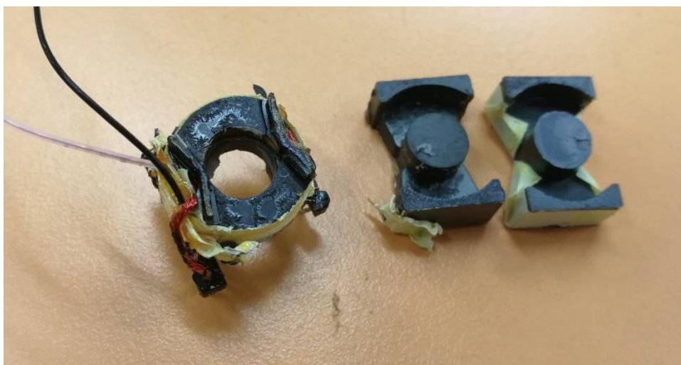
Exploded view of transformer
