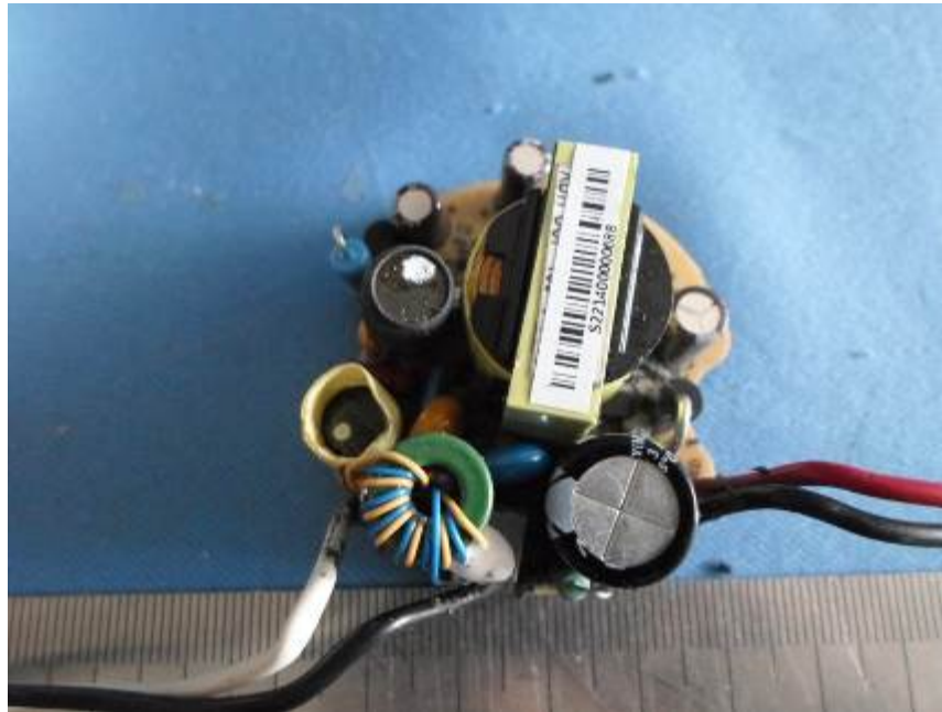
Fig. 11 – internal of EBR020E-0500-42
