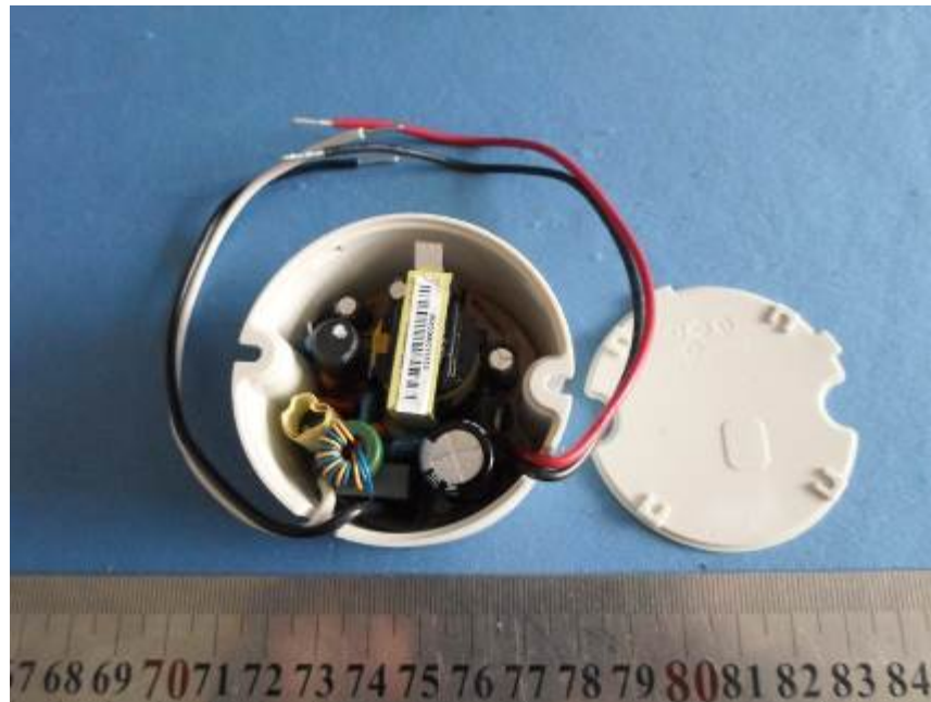
Fig. 19 – PCB of EBR010W-0250-42
