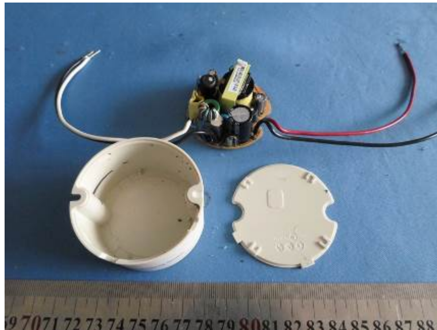
Fig. 15 – internal of EBR020W-0400-42
