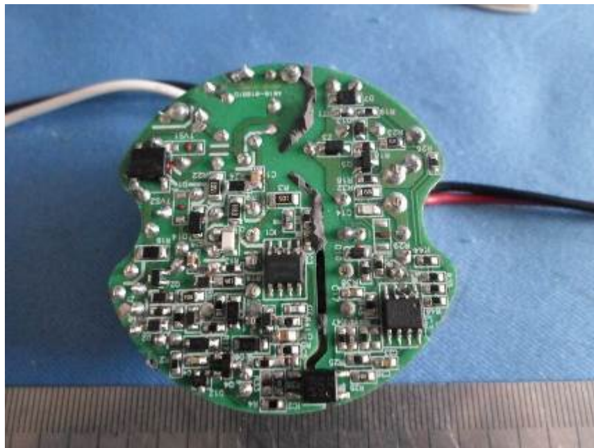
Fig. 12 – internal of EBR020E-0500-42
