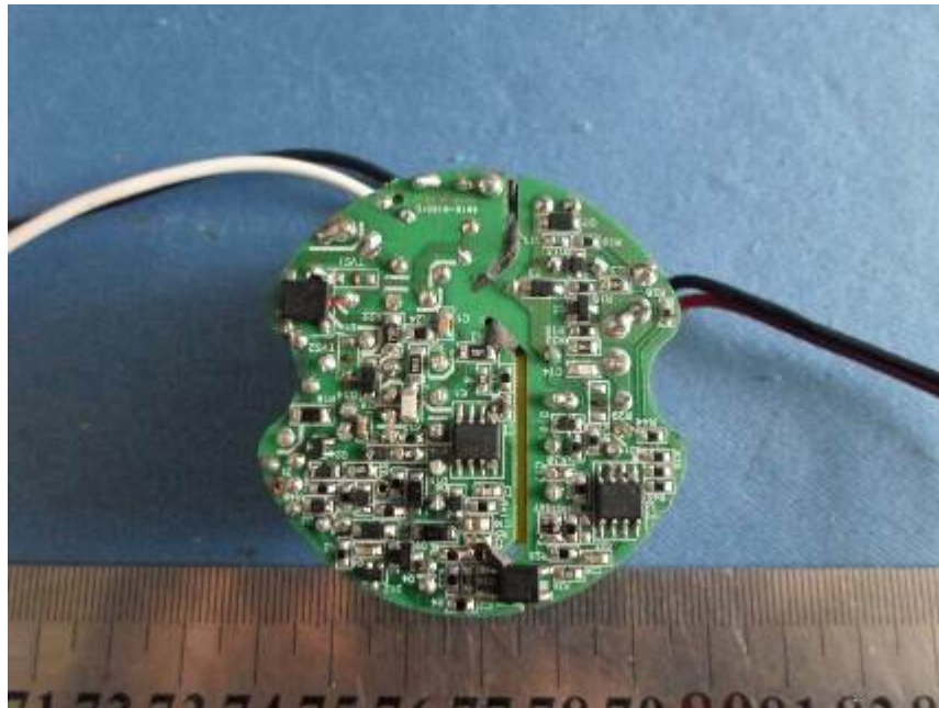
Fig. 6 – internal of EBR020E-0700-30
