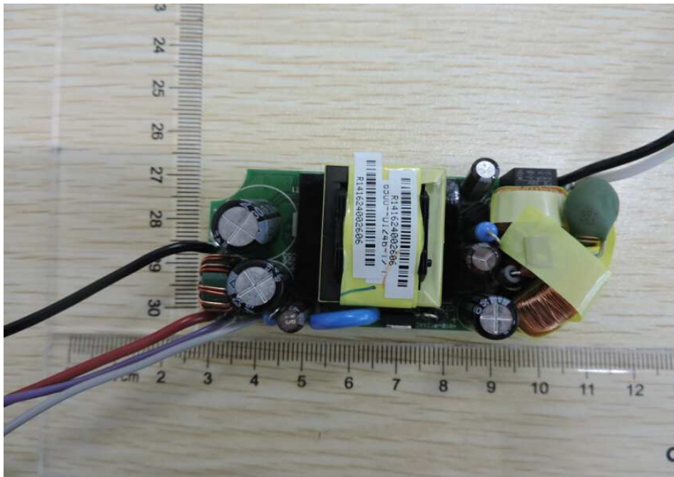
Picture 9: Top view of PCB for ESS series models
