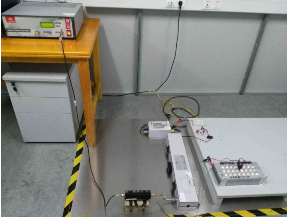
Photograph 6: Set-up for Radio-Frequency Electromagnetic Field (RS)
