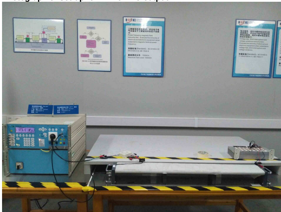
Photograph 8: Set-up for EFT on DC output
