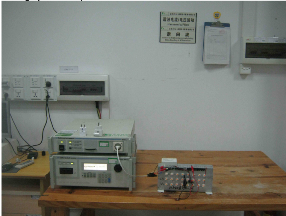
Photograph 2: Set-up for Disturbance Voltage AC Mains:
