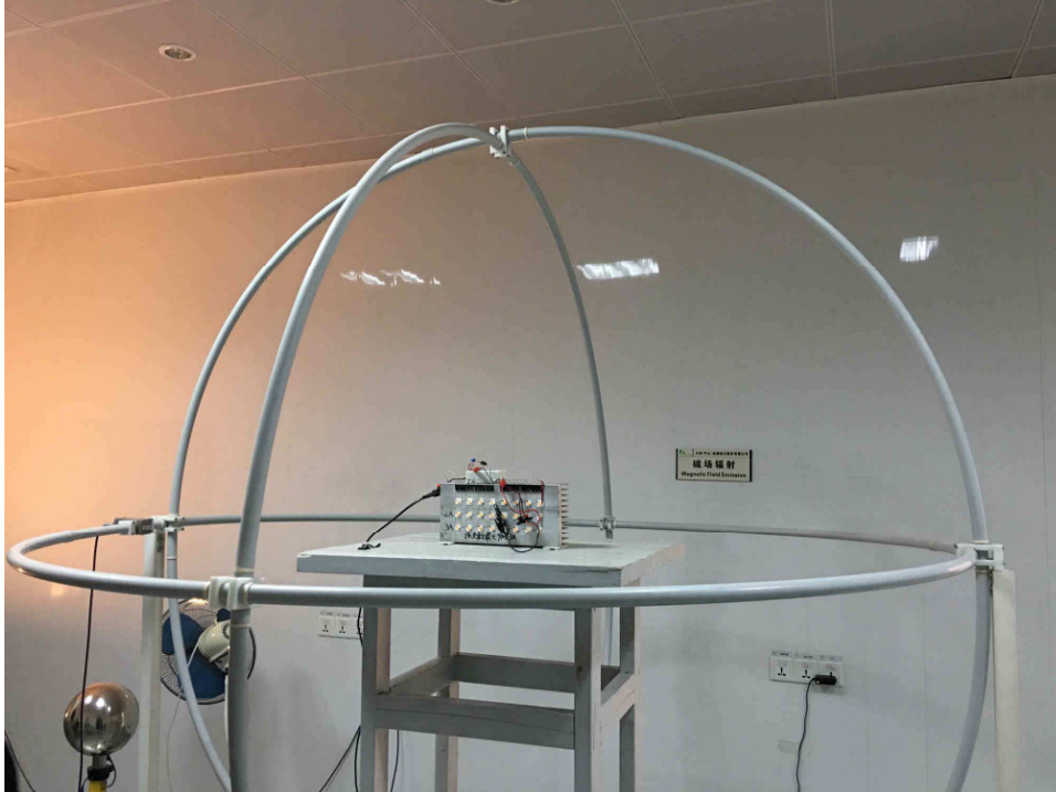
Photograph 3: Set-up for Radiated Electromagnetic Disturbances (Table 3a)
