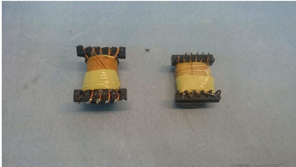
Picture 13: Primary winding was isolated from Secondary winding by insulation tape
