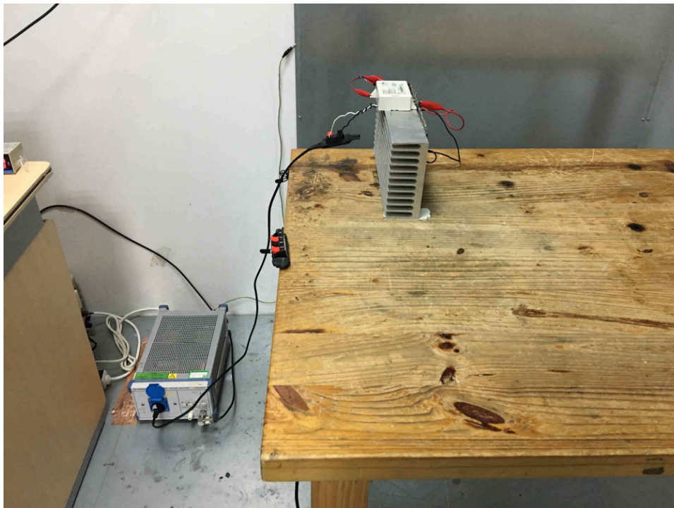
Photograph 2: Set-up for Disturbance Voltage AC Mains:
