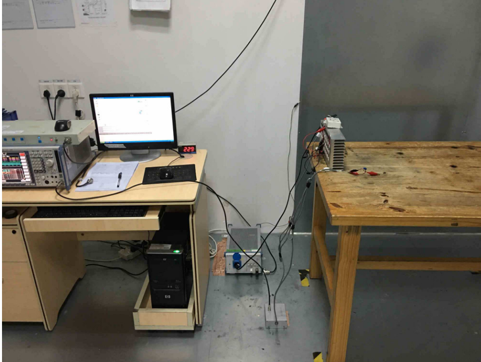
Photograph 3: Set-up for Radiated Electromagnetic Disturbances (Table 3a)
