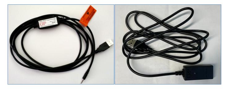
The USB-JACK cable, provided for configuring Draco LED drivers, uses a USB port to connect to a computer, and a proprietary barrel jack connector, to interface with the Draco LED driver. The NFC cable, provided for configuring NFC series of drivers, uses a USB port to connect to a computer and an NFC wand to interface with NFC series of drivers.
